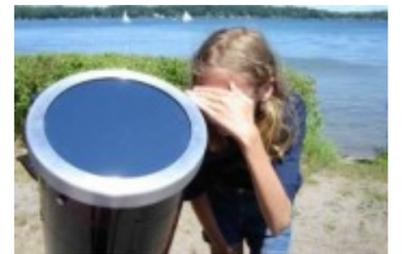
Note #1: The sun's immense energy must be drastically reduced *before* it enters the telescope. Do not use small filters that fit over the eyepiece (as found in some older, cheaper telescopes), for the concentrated sunlight can shatter them.
