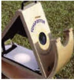
The **Sunspotter** is commercially available from Science First. It provides a surface on which you can safely trace the sun's outline and sunspots onto a piece of paper.
