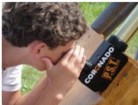
Special telescopes with built-in hydrogen-alpha filters show additional solar features, such as the sun's surface granulation and prominences extending outward into space. Though more expensive than traditional telescopes, they offer wonderful views of the magnified sun not seen by astronomers in previous centuries.
