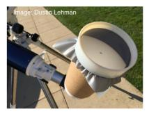
◆ You can also 3D-print both an end ring to hold the projection screen and an eyepiece holder that slide over each end of a 5-inch diameter tube. For 3D printer files, see http://tinyurl.sun3D.
