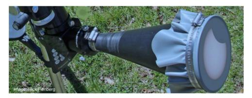
You make a Sun Funnel by clamping a piece of rear projection screen material over the large end of a plastic funnel and clamping an eyepiece into the narrow end of the funnel. Then insert the eyepiece barrel into your telescope focuser.
